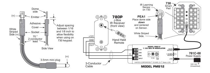
**Fig. 3** The PEA1 Programming Emitter Assembly (included with PMS12)
